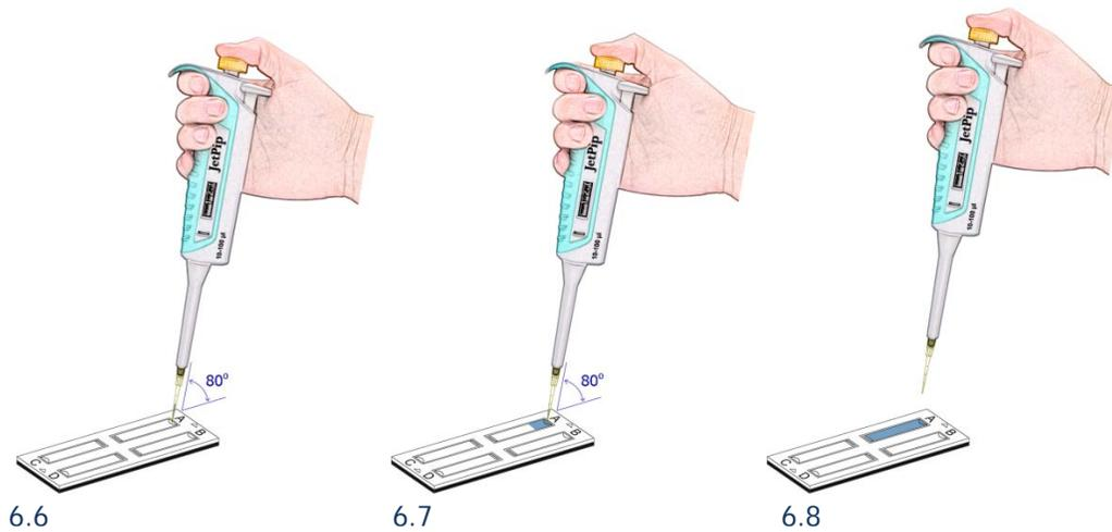
In order to load the rest of the micro-fluidic cameras of the LACTOCHIP x4, repeat the procedure described in points 1 to 6 by consecutively filling the micro-fluidic cameras from A-D.
