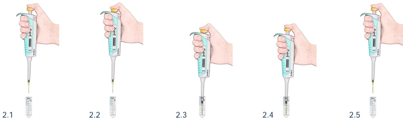
Pipette milk in the opened micro-tube on the rack by smoothly pressing the working button of the pipette from the initial position to the first stop (see 2.6, 2.7). After a short period press the button to the second stop (see 2.8). In this way you'll empty the tip and will guarantee precise pipetting. Always pipette the milk without dipping the tip in the lyophilized dye.
